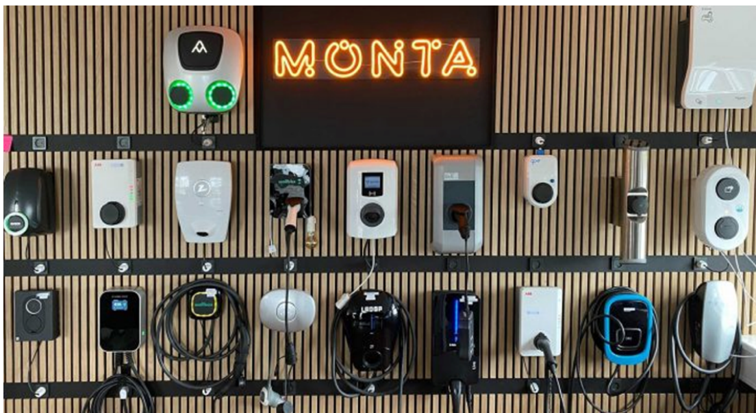
Figure 2 A wall full of different EVSEs on display at the site of charging settlement back-end operator, Monta, illustrating differences in mechanical design of the box, but all with same basic functionality. There can be small variations between boxes in the level of remote charge control available [1]
